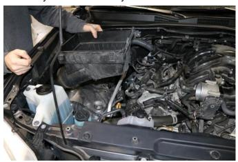
**8.** Remove three 12mm mounting bolts using a ratchet and 12mm socket. There are two mounting bolts inside of the box and one is behind the box. Remove factory air box from vehicle. Save two mounting bolts for Install Step 3.
