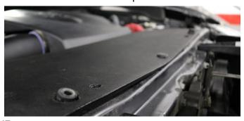
**15.** Use clip from **Install Step 12** to secure scoop.
