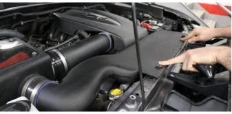
**14.** Attach straight sleeve onto air box and slide scoop into place over hood rubber stops.
