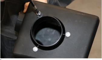
Install filter adaptor onto Volant air box with provided hardware using a ratchet and 10mm socket.
