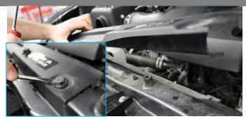
**12.** Remove 7 retaining clips using pry tool. Save 1 clip for Install Step 15. Remove tray cover.
