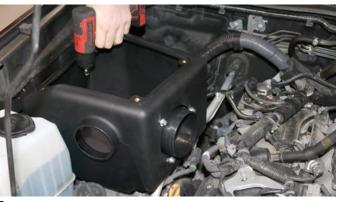
Insert Volant air box into vehicle and mount using two of the bolts from Removal Step 8 of removal. Use a ratchet and 12mm socket to mount box to factory location.
