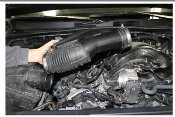
**6.** Remove factory air duct.
