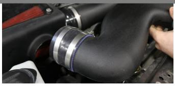
**13.** Place two #56 clamps and straight sleeve onto the Volant RAM Air Scoop.
