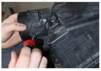
**9.** Using a Philips head screwdriver, remove MAF sensor from stock lid.
