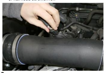
9. Re-attach MAF sensor wire.
