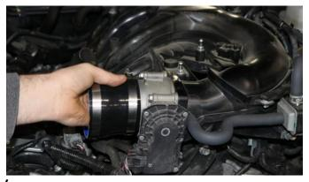
Insert two #56 clamps on reducer, and place small end of the reducer on the throttle body.
