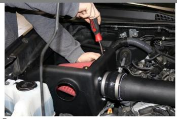
7. Insert filter with clamp into box, and onto filter adaptor, making sure filter is fully seated on adapter. Tighten using a ratchet and 8mm socket or flat head screwdriver.
