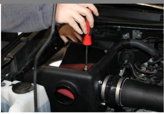
**8.** Install Volant lid onto air box, secure with provided four truss head screws with rubber washers using a Philips head screwdriver.
