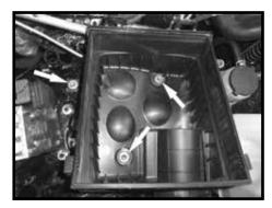
Step 5 Remove the three bolts securing the bottom of the air box to the vehicle then remove the bottom of the air box.
