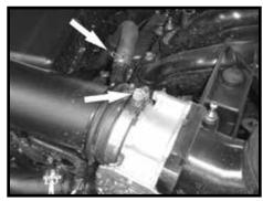
Step 3 Loosen the hose clamp that secures the intake tube to the throttle body. Disconnect the breather hose at the intake tube.
