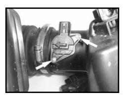
Step 7 Remove the two screws securing the mass air meter sensor to the stock intake tube and then remove the sensor.
