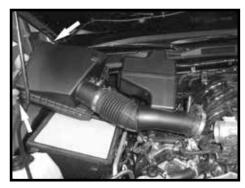
Step 4 Release the two clips securing the top of the air box and remove the air box intake tube assembly from the vehicle. Remove the stock air filter.
