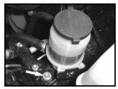
Step 6 Remove the bolt that secures the power steering reservoir to the vehicle. The screw will be reused in step 10.
