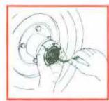
Install clutch assembly. Cross torque allen screws to 14-16 Kp. cm (12-14 in. lbs).
