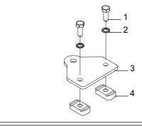
Locate the work light bracket to the top recess of the crossbar.
