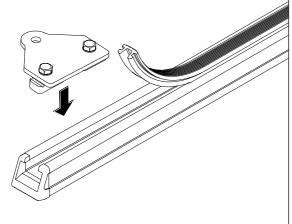
Locate the channel nut into the crossbar recess, turn the attachment bolt so that the channel nut rotates and locates across the crossbar. Adjust the position of the bracket and tighten the attachment bolt. Check that the channel nut is fully located across the crossbar after tightening. Trim rubber buffer strip to suit.
