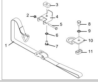
Insert the camlock and hook bracket onto the underside recess of the crossbar. Push the attachment bolt up and turn the bolt so that the channel nut is fully located across the crossbar as per the diagrams. Position the camlock and hook bracket to suit the ladder, tighten the bolts.
