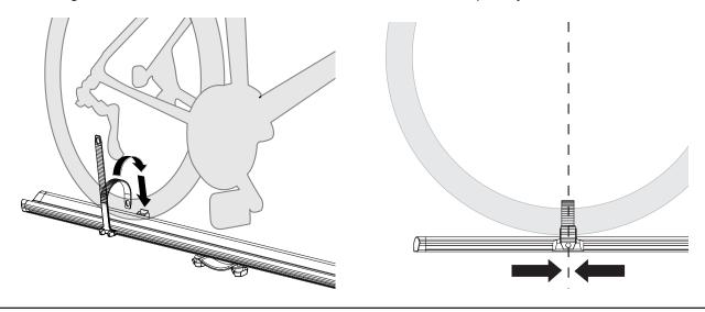
The Quick Release Skewer is not an on/off switch. You must close the handle with enough tension to hold the bicycle. Rock the bicycle side to side to ensure proper mounting. The fork should be properly seated and not move. If unsure, please consult your dealer or Rhino-Rack. Failure to comply could result in the bicycle detaching with subsequent damage to the bicycle, vehicle, or other motorist
