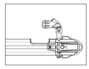
Open the handle of the quick release so the black handle is straight and the fixed end points down. Load the fork onto the quick release so both fork ends are resting straight on the quick release.
