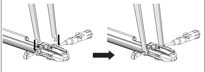
Twist handle clockwise to tighten the quick release skewer. Close the handle by flipping it 90 degrees to the closed position. If it is too loose, open the handle and turn it like a screwdriver (clockwise to tighten, counter clockwise to loosen), and close the handle again. Re-adjust until a firm and positive snap is felt when closed. If locks have been purchased or provided, the cover can now be locked.
