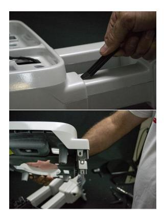
6. You will now have access to the light. Remove it from the assembly and install the RECON light in its place and reassemble the mirror housing.
