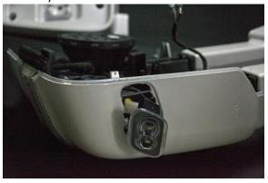
5. Next, release the three clips on the top of the mirror assembly and pry the two arms to separate the trim and gain access to the light assembly.
