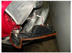
Using A Sealant, Apply A Liberal Amount To Protect Exposed Connectors
