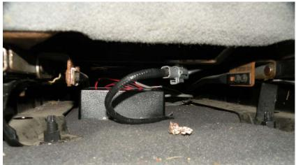
Based Off of Chart Below Determine The Size Of Wire Used To Power & Ground The Power Supply. Be Sure To Install A Fuse (Not Included In this Kit) Within 1 Foot Of 12V+ Connection To The Battery.
