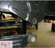
9. Support the transmission cross member with a suitable jack stand. Working on one side at a time, unbolt and remove two transmission cross member bolts.
