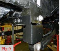
11. Rotate the axle and install the radius arms into the drop brackets using 18mm x 130mm bolts, washers and c-lock nuts. Do not tighten at this time.
