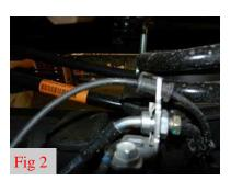
4. Locate the 2 brake line/ABS brackets attached to the axle and remove brackets.
