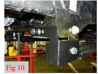
12. Torque the cross member bolts to 165 ft-lbs. Torque the factory 18mm hardware to 285 ft-lbs. Leave the radius arms loose. They will be torqued once the vehicle is on the ground.
