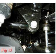
17. Lower the axle enough to remove the front springs. Make sure to not over extend the brake/ABS lines. (Fig 14)
