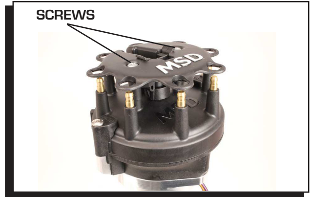
Figure 11 Installing the Wire Retainer
