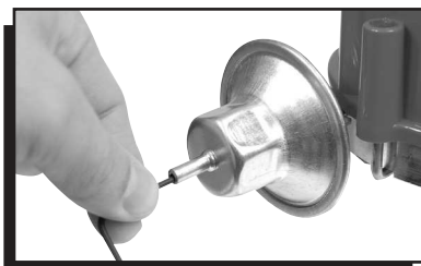
Figure 2 Adjusting the Vacuum Advance.
