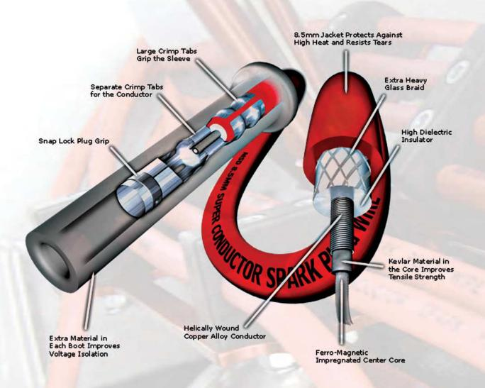
The 8.5mm Super Conductor wire is the best wire you can run on your engine whether it's a cruiser, sport compact or all-out race car. With less than 50 ohms per foot resistance, you can ensure that the most spark energy possible reaches the spark plug gap. More spark energy means improved combustion resulting in increased performance!
