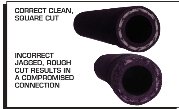
Figure 5 Severing the Hose Properly.
