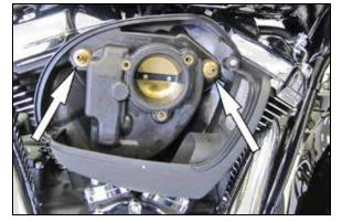
4. Remove the two breather bolts shown and then remove the rear air filter housing from the vehicle. NOTE: K&N Engineering, Inc. recommends that customers do not discard the factory air intake components..
