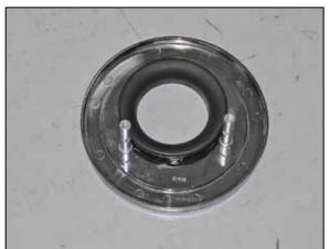
10. Install the two provided spacers onto the filter back plate and secure with the provided hardware. NOTE: Apply one drop of the provided thread locker to the threads of each bolt.
