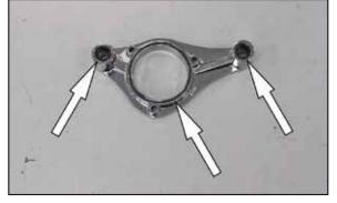
7. Install two of the breather O-rings and the throttle body O-ring into the base plate as shown. NOTE: Use a few small dabs of grease to secure the O-rings in place while installing the base plate to the engine.
