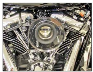
11. Install the filter back plate assembly onto the base plate and secure with the three throttle body bolts provided.
