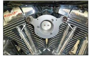
9. Using the two provided crankcase breather bolts install the back plate onto the vehicle as shown. Do not tighten the breather bolts at this time.
