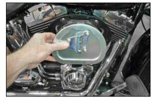
4. Remove the air filter with breather hoses as shown.
