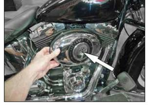
2. Remove the air filter cover retaining bolt and then remove air filter cover as shown.
