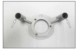
7. Install two o rings provided onto the back side of the K&N $^{\odot}$  back plate as shown.
