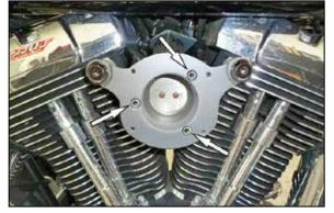
10. Install the provided gasket between the throttle body and back plate use the provided hardware to secure the back plate to the throttle housing. Tighten the crankcase breather bolts. **NOTE: Apply one drop of the provided thread locker onto the provided bolts.**
