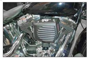
12. Install air filter and air filter cover with provided bolts.
