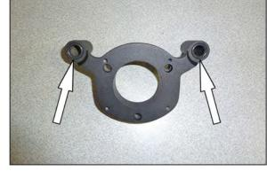
8. Install the remaining two o rings onto the front of the back plate as shown.
