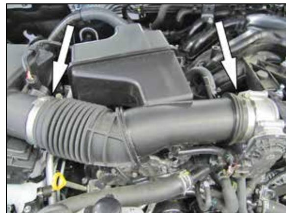
4. Loosen the two hose clamps securing the factory intake tube and then remove the intake tube from the vehicle.
