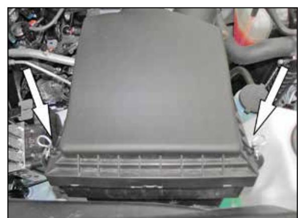
5. Release the two clips securing the upper air filter housing and then lift up the housing and remove the factory air filter.
