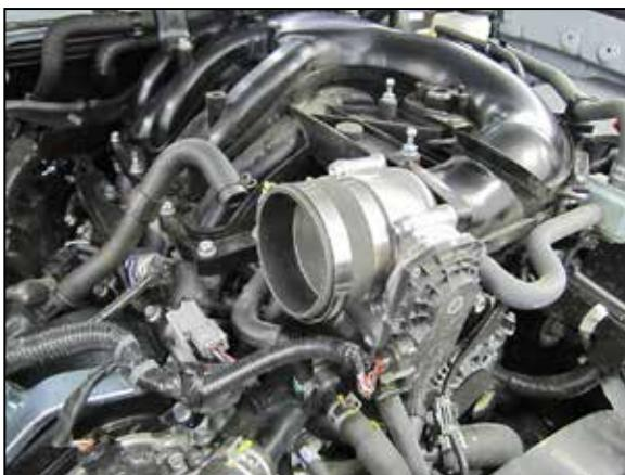
8. Install the provided coupler hose (08690) onto the throttle body and secure with the provided hose clamp.
