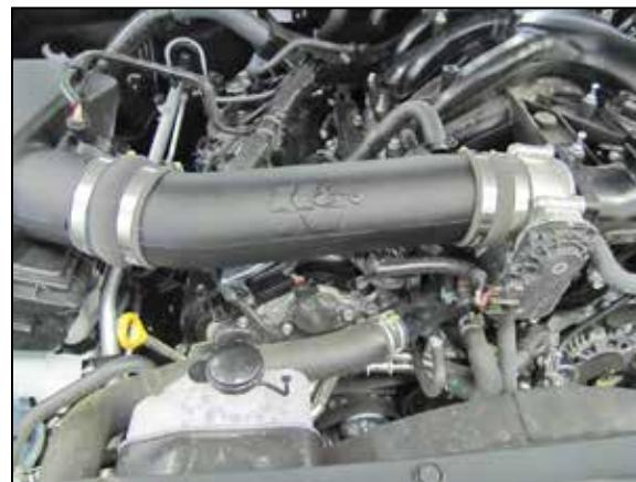
10. Install the K&N® intake tube into the hump coupler at the air filter housing lid and then into the coupler at the throttle body, resecure the air filter housing lid, adjust the tube for best fit and then secure the hose clamps.
