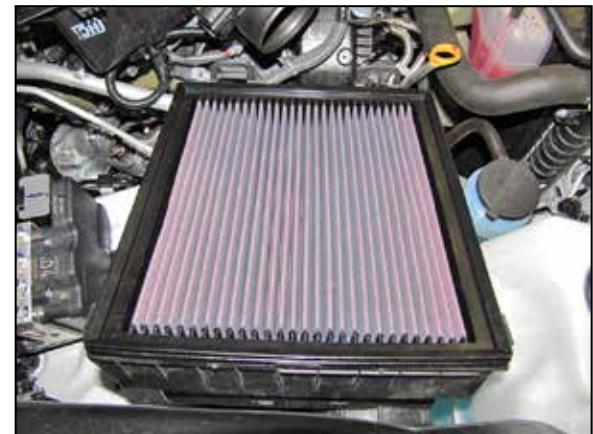
6. Install the K&N® air filter into the lower air filter housing and then reinstall the upper housing. Do not secure the lid at this time.
