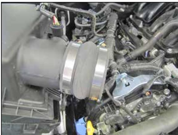
7. Install the provided hump coupler (08171) onto the factory air filter lid and secure with the provided hose clamp.
