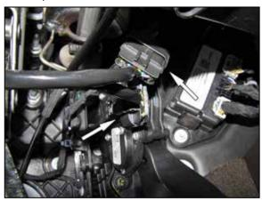
3. Connect the K&N® throttle wiring harness to the throttle pedal and connect the factory wiring harness to the K&N® wiring harness.
