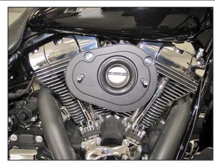
8. Install the back plate along with the two remaining O-rings, breather bolts, and throttle body mounting bolts as shown.
