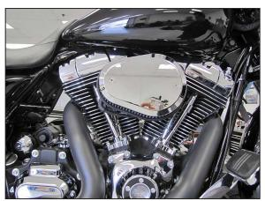
Install the filter and top plate onto the back plate and secure with the provided hardware.
