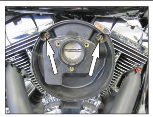
4. Remove the two crank case breather bolts shown and then remove the air filter base from the throttle body.
