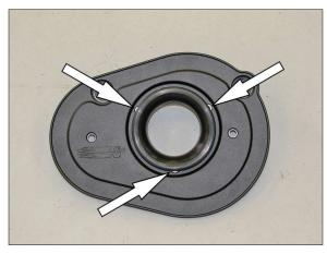
5. Install the provided venturi and the three throttle body mounting bolts into the back plate as shown. NOTE: The bolts pass through the back plate and venturi on the back side.
