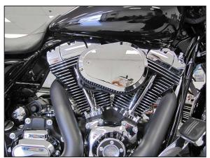
Install the filter and top plate onto the back plate and secure with the provided hardware.
