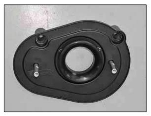
6. Install the two provided spacers onto the back plate as shown using the provided hardware.
