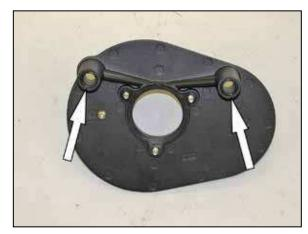
7. Install two of the provided O-rings into the crank case breather plate as shown.
