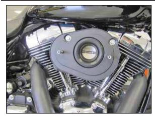
8. Install the back plate along with the two remaining O-rings, breather bolts, and throttle body mounting bolts as shown.
