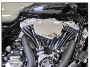
9. Install the filter and top plate onto the back plate and secure with the provided hardware. NOTE: be sure to place one drop of thread locker to the mounting bolts.
