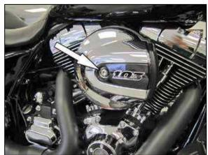
2. Remove the bolt which secures the bonnet to the filter assembly and then remove the bonnet from the vehicle. **NOTE: On some applications the engine cubic inch badge may cover the bolt, the badge is held on with Velcro. Peel the badge off to expose the bolt.**
