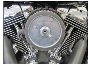
9. Install the filter onto the base plate and secure with the provided hardware.NOTE: be sure to apply one drop of thread locker to each bolt.
