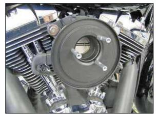
7. Install the filter spacer bolts through the filter back plate and then install the gasket onto the spacer bolts passed through the back plate. Install the filter back plate assembly onto the breather plate and secure with the filter spacer bolts. **NOTE: Be sure to place one drop of thread locker on each bolt.**
