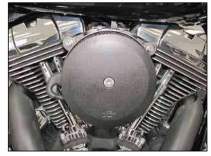
10. Install the filter cover plate onto the filter and secure with the provided hardware. NOTE: be sure to place one drop of thread locker to the cover plate mounting bolt.
