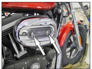
2. Remove the bolts securing the air filter bonnet and then remove the bonnet.
