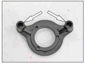
6. Install two of the provided O-Rings into the K&N® throttle body bracket as shown.
