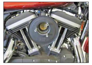
8. Install the filter back plate and secure with the filter spacer bolts.
