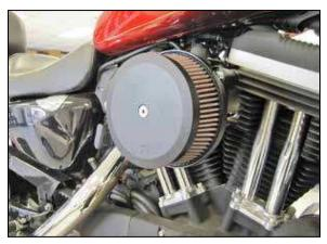
11. Install the filter cover and secure with the provided bolt.
