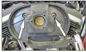
4. Remove the O-Rings from the breather bolts and then remove the breather bolts and rear air filter housing.
