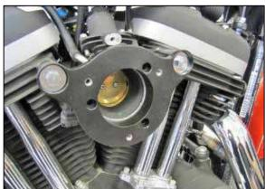
7. Install the two remaining O-Rings into the front side of the K&N® throttle body bracket, then insert the two provided breather bolts through and attach the assembly to the cylinder heads but do not completely tighten. Insert the provided throttle body gasket and then install the filter spacer bolts to hold the gasket in place. Tighten the breather bolts and then remove the filter spacer bolts.
