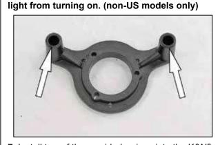
7. Install two of the provided o-rings into the K&N® crankcase breather plate as shown.
