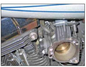
6. On Models equipped with the electrical pigtail, using the provided tie wrap, secure the wiring pig tail to the throttle body wiring harness.
