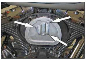
3. Remove the three bolts which secure the air filter to the filter base and then remove the air filter along with the crank case breather tubes.
