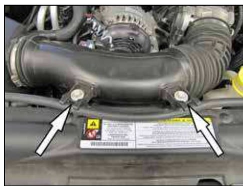
3. Remove the two bolts which secure the factory intake tube to the fan shroud.
