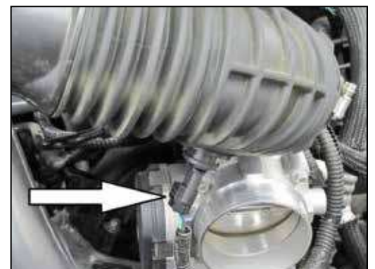
6. Lift up the intake tube, disconnect the inlet air temperature electrical connection then remove the intake tube from the vehicle.
