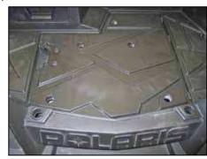
23. Reinstall the engine access panel.
