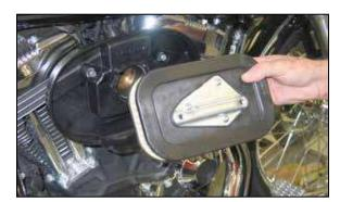
4. Remove the air filter as shown.
