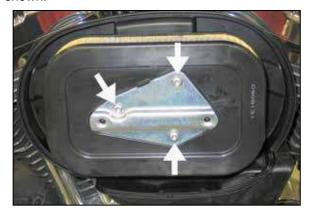
3. Remove the three air filter mounting bolts shown.
