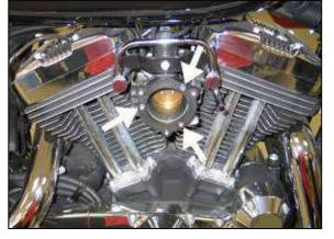
8. Install the K&N® intake tube adapter onto the throttle body using the provided hardware. NOTE: Apply one drop of the provided thread locker to the three tube adapter mounting bolts.
