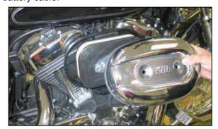
2. Remove the two air filter cover mounting bolts and then remove the cover from the vehicle as shown.
