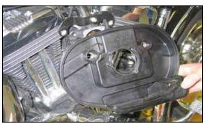
6. Remove the air filter base as shown.
