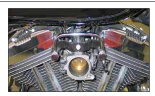
7. Install the K&N® crankcase breather tube onto the vehicle using the provided hardware. NOTE: Do not completely tighten the breather bolts at this time.
