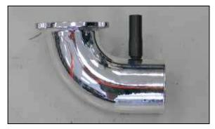
9. Cut the provided crankcase vent hose to a length of 1.75" and install onto the K&N® intake tube as shown.
