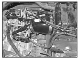
9. Reconnect the fuel injection electrical connections.
