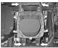
15. Remove the four air box mounting bolts shown.
