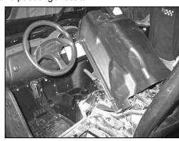
3. Lift up the engine cover and remove it from the vehicle as shown. It will be necessary to push the shifter boot through the engine cover as it is removed.
