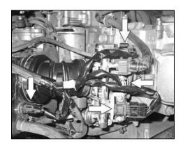
4. Unhook the four fuel injection electrical connections shown and place the wiring harness to the side away from the intake hose.
