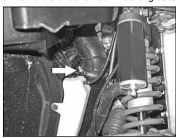
16. Loosen the hose clamp which secures the intake tube to the lower air box.
