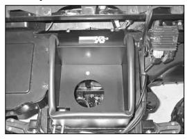
21. Install the heat shield assembly into the vehicle and secure with the provided hardware to the factory air box mounting locations.
