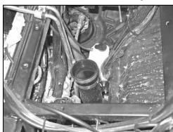
18. Install the provided silicone hose (08434) onto the intake tube and secure with the provided hose clamp.
