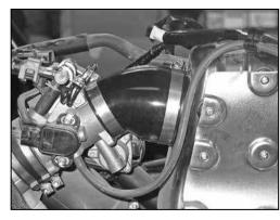
8. Install the silicone hose assembly onto the throttle body and air chamber and secure with the hose clamps.
