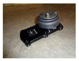
The shifter "body" will be in the rear position on the rear TKO shifter cavity. Make sure the pivot ball is positioned into the rear socket and that the white plastic bushing is still in place.
