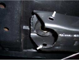
Weld-in: Grind/sand near the designated area marked earlier on the front subframe.
