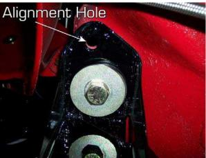
3 – The subframe connectors must be installed on an alignment rack or floor ramps (all 4 wheels). The vehicle must be sitting on it's wheels at ride height in order to install the subframe connectors. Do not use a two-post lift, as this will load the chassis/body in the wrong points causing the chassis to tweak.
