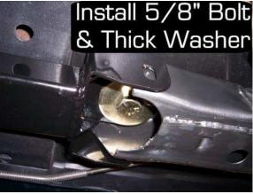
Bolt-In: Mark the front subframe to indicate where your bolt holes will be.
