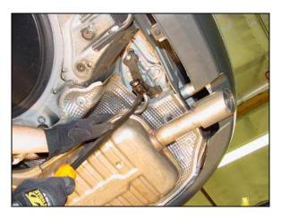
4/ Remove the two lower end link bolts (16mm wrench) which attach the sway bar ends to the end links. You may need to hold the wrench-flat with a 17mm wrench.
