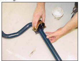
6/ Lift the bar up to the vehicle with the two smaller H-Sport stickers at the ends right-side-up. As you lift the bar up to the mounting points, <u>you must place one mounting plate per side between the bushing and the mounting point.</u> This relocates the bushing out of the stock bushing pocket. Re-install the bracket nuts and tighten. <u>Re-install the end link bolts and tighten well using medium strength thread locker</u>.
