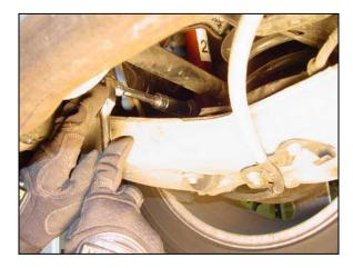
5/ Remove the four bushing bracket bolts (13mm wrench) attaching the antiroll bar brackets to the sub-frame and save them.
