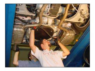
7/ Repeat same pressure to the exhaust and position Hotchkis bar (without the bushings and brackets) in the stock location with the Hotchkis sticker facing
