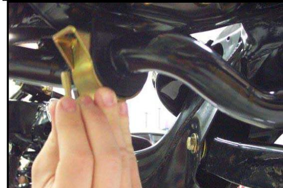
11. Install the new A-Arm endlinks using a ratchet and wrench.
