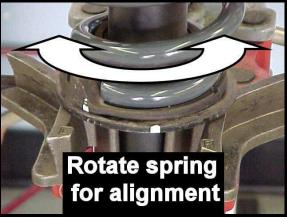
13) Once aligned, compress the coil spring and install the shaft nut back on. Fully tighten hardware.
