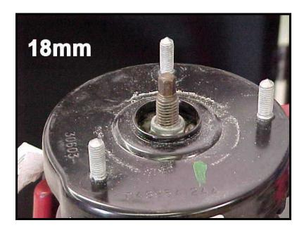
9) Remove the top hat, stock bumpstop, and stock spring at this time. Sometimes the bumpstop is pressed into the top hat, in which case, remove the stock bumpstop from the top hat boot.
