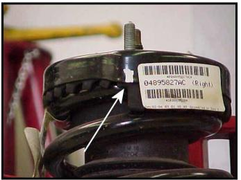
8) Secure the spring/shock assembly in your spring compressor and remove the shaft nut using a 18mm socket. Retain hardware for reinstallation.
