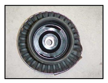
11) Place your new Hotchkis coil spring onto the shock. Make sure the smaller pigtail end is on the bottom.
