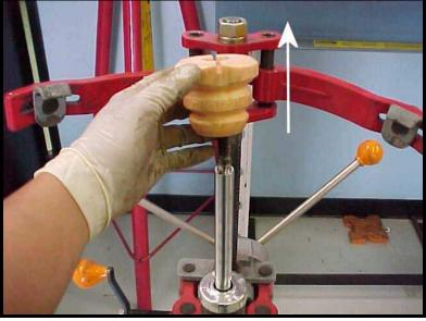
10) Place your new Hotchkis polyurethane bumpstop into the top hat boot assembly as shown in the picture.
