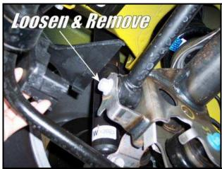
3 Detach Passenger Side End: Locate the passenger side panhard rod end and loosen & remove the mounting bolt. Retain stock hardware for later use.
