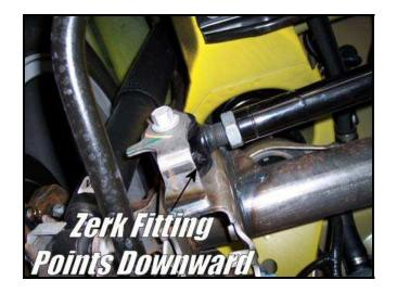
8 Attach Passenger Side: Reuse the stock hardware to fasten the passenger side mount. The axle might be slightly shifted from the body, so it may be necessary to use a pry bar to line up the mounting hole with the panhard rod hole. Once the bolt is started, fully tighten both driver and passenger side bolts.
