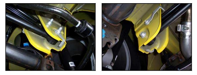
4 Remove Panhard Rod and Compare to Hotchkis: Lay the stock panhard rod next to the Hotchkis rod and adjust the Hotchkis rod to the same length. This will give you a good starting point.
