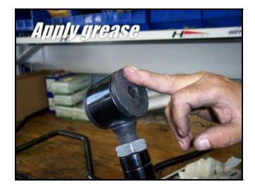
6 Install Hotchkis Panhard Rod: Insert the Hotchkis rod in same manner as stock removal.
