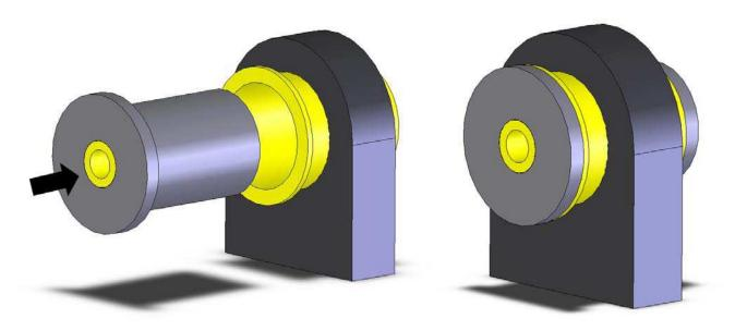
13. Install the thrust washer onto the unflanged side of the can.
