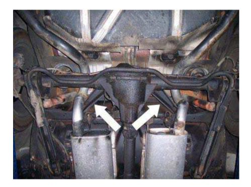
Now here comes the difficult part; removing the stock Can Bushings. These are the bushings that connect the aft end of the upper trailing arms to the differential. You may luck out and be able to hammer them out with a dead blow hammer, but if you are not able to use this method please do the following.
