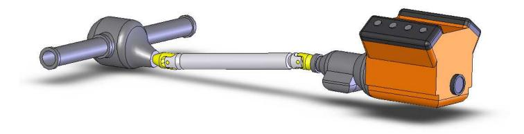
The Hotchkis double adjustable trailing arms allow you to adjust the pinion angle with ease. Simply loosen the two jam nuts and rotate the aluminum turnbuckle to lengthen or shorten the arm. So, how does one set the pinion angle?
