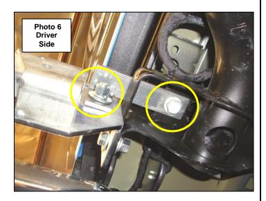
**Step-10** With assistance attach the bumper shell brackets to each frame bracket using (2)  $\frac{1}{2}$ " x 1  $\frac{1}{2}$ " hex bolts, (4)  $\frac{1}{2}$ " flat washers, (2)  $\frac{1}{2}$ " lock washers and (2)  $\frac{1}{2}$ " Hex nuts, Align the bumper shell with the vehicle, verify that the tailgate clears when lowered, and tighten all nuts and bolts, (Photo 7). If necessary, loosen the frame / receiver hitch bolts to adjust the bumper shell.
