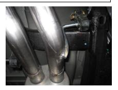
4.Next install passenger side overaxle tailpipe #C into muffler 1.5" to 2" insert welded hanger into rubber grommet use clamp # F to secure pipe to muffler do not tighten
