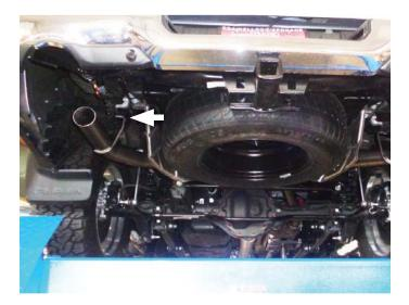
15. Place **tips (x2) (ST462B)** onto left exit and right tailpipe. Tighten nut on tips to fully install them.
