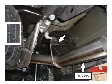
13. Connect left **over-axle (26730S)** to muffler and hang wire hanger in stock isolator. Tighten clamp just enough to allow for adjustment.
