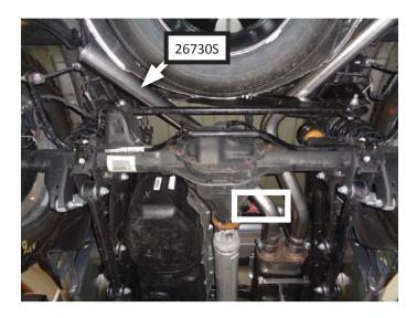
14. Place **clamp (MC300BS)** onto **left exit (26731S)** inlet. Connect left exit to left over-axle and hang wire hanger in stock isolator. Tighten clamp just enough to allow for adjustment.
