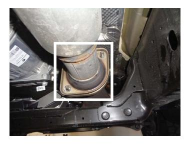
7. Remove muffler and factory pipe from vehicle.
