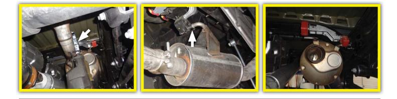
5. Remove factory muffler wire hangers (x3) from factory isolators and detach grounding wire.
