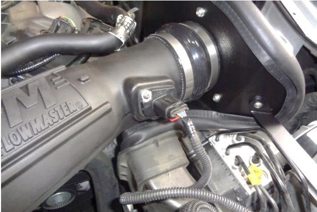
31. Plug the MAF sensor lead into the sensor, push the latch in, and verify the connector is secure.
