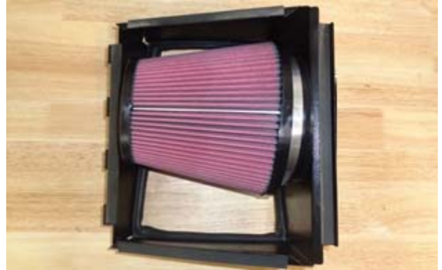
16. Slip screw clamp (2) onto the air filter (1), install the filter on the filter adapter, and tighten the clamp.
