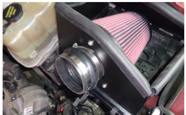
18. Slip a #56 screw clamp (6) onto the small end of the straight coupler (7), and install the coupler on the filter adapter. Push the coupler up against the heat shield and tighten the clamp. Then slip a #64 screw clamp (20) over the other end of the coupler.
