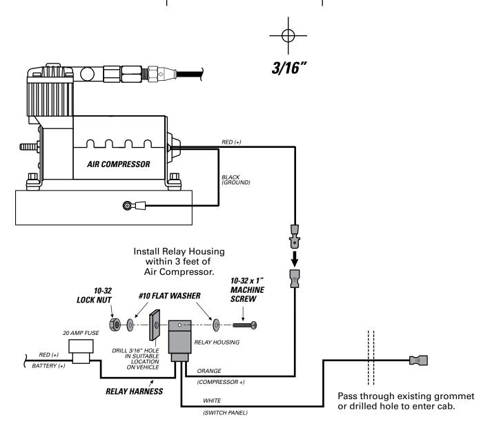
Connect wires, install Ring Terminals and Wire Connectors as shown below. **2** Fasten Control Panel ground wires to vehicle as shown.
