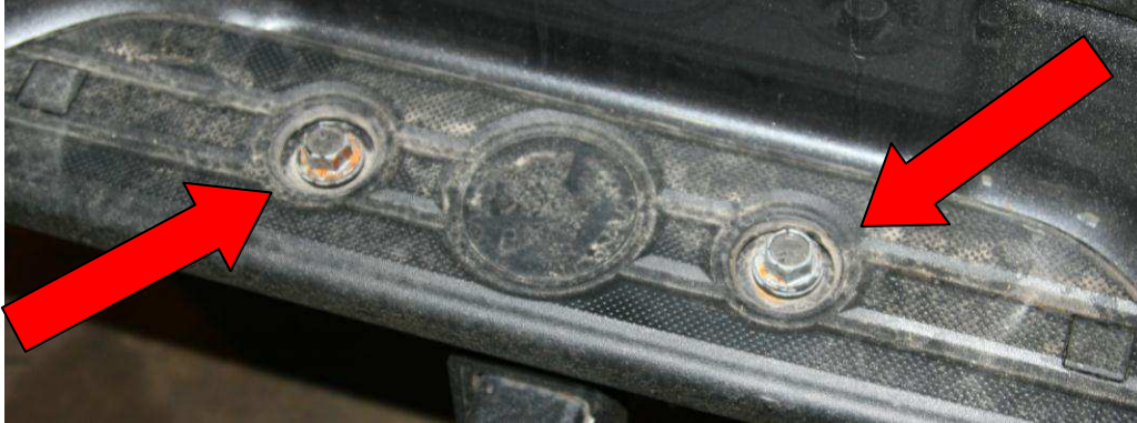
Figure 3 – Trailer hitch bolt removal
