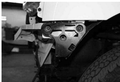
Figure 4 - Spacer Fastener Locations
