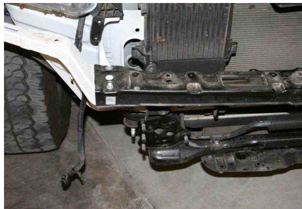
Figure 3 – BUMPER TO FRAME FASTENER REMOVAL
