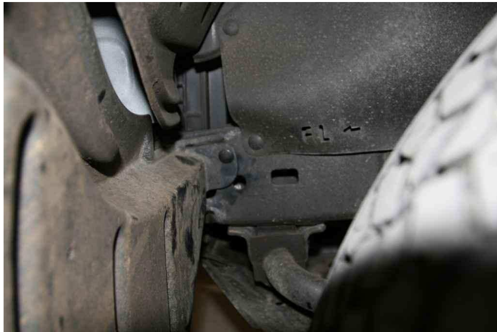
Figure 1 – FENDER LINER DART CLIP REMOVAL
