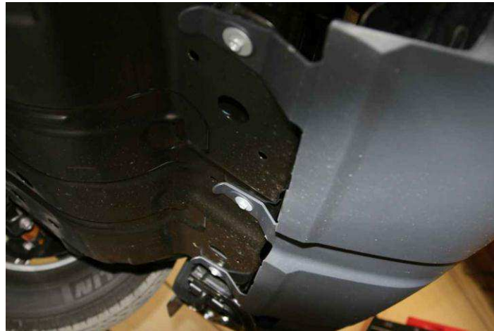
Figure 2 – LOWER BUMPER PLASTIC REMOVAL
