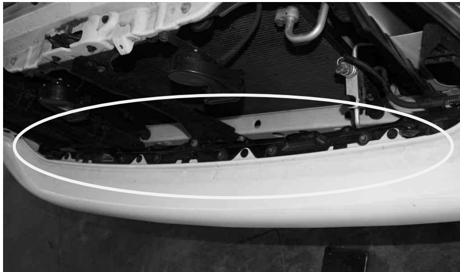
Figure 2 - Center Fascia Fasteners
