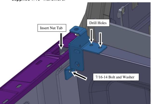
B. With Bracket installed to the bedsides drill the holes into the top of the bulkhead with a  $\frac{1}{2}$ " Drill Bit. Install supplied 7/16" Hardware using the Double Nut Tab using your finger in the loop to align it through the gap between the bed and the cab.
