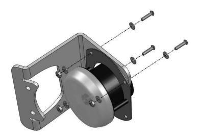
H. Install the fog light and bracket into the bumper using the remaining two holes available in the light insert. Use the 1-1/2" length 1/4" stainless steel button heads with 1/4" washers and nuts.
