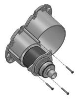
F. Install the light inserts with turn indicators into the cutout in the bumper. Use the <sup>3</sup>/<sub>4</sub>" length <sup>1</sup>/<sub>4</sub>" stainless steel button head, <sup>1</sup>/<sub>4</sub>" washers and hex nuts to fasten the insert through the holes shown below:
