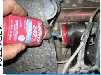
Use a wire brush to remove any remaining old rubber. File off any sharp edges that will contact the new polyurethane bushings. Apply grease to all metal parts that contact the polyurethane bushings. Apply thread locking compound to upper control arm through bolt then torque to 85 ft. lbs.
