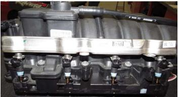
16. Remove the eight (8) injector retaining clips and pull the injectors out of the rail. **NOTE:** The fuel injector clip can be removed by pushing the clip inward (toward the manifold).
