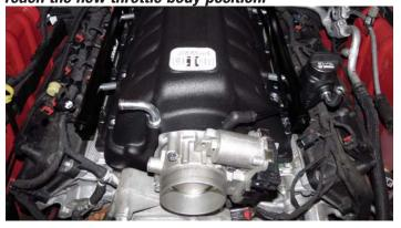
35. Reconnect the EVAP hose to the fitting on the driver side front of the manifold.
