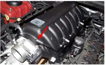
36. Using appropriate fuel and oil resistant hose (not included), connect the PCV on the passenger side rear of the manifold to the fitting on the passenger side front of the manifold.
