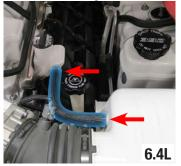
3. Loosen the worm clamps securing the air inlet tube to the airbox and throttle body. Disconnect the engine harness from the IAT sensor and remove the air inlet tube. Using a 8mm socket, remove the bolt securing the stock airbox and remove the airbox.
