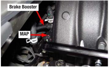
30. Reposition the intake manifold on the cylinder heads so the mounting holes on the manifold line up with the corresponding holes on the cylinder heads.
