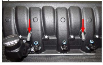
26. Install the fuel rails with injectors onto the manifold making sure the fuel rail spacers stay in place. Firmly and evenly press down on the rails until the injectors are fully seated into the manifold.
