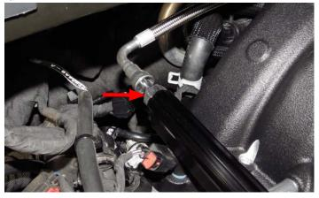
41. Install the provided fuel rail crossover to the 3/8" male fittings installed during step #40.
