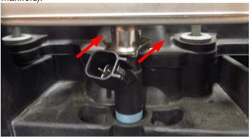
17. Remove the MAP sensor from the factory intake manifold and set aside. On 6.1L and 6.4L engines the bolt(s) retaining the MAP sensor must be removed. On 5.7L engines the MAP sensor is twist locked into place. (6.4L shown; Use Torx 20 to remove bolt)
