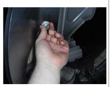
6. Torque 1/2" hardware to 110 lb-ft and M12 hardware to 79 lb-ft.
