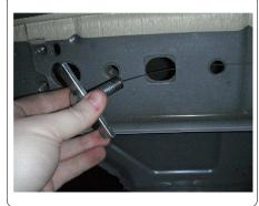
5. Raise hitch into position by placing passenger side of hitch over the passenger side muffler first and then raise the driver side of hitch. Secure hitch to existing weldnuts with supplied M12 hardware and conical toothed washers. Attach 1/2" hex flange nuts onto carriage bolts.
