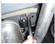
2. Locate and remove (2) rubber isolators from exhaust pipe.
